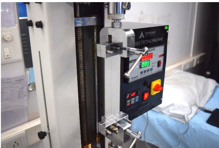
Figure 7: Hair Tensile Strength Measured with TESTRONIX
